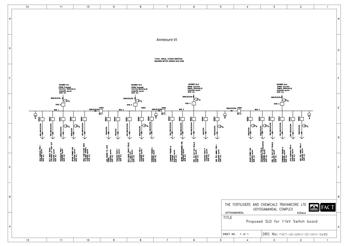
CLOSE BC-1 RTC- Ready to Close CLOSING LOGIC: BC-1 I<sub>2</sub> OFF PI I3 OFF I<sub>2</sub> OFF P1 L OFF I, OFF L OFF BC-2 OFF BC-2 ON BC-3 OFF р **BC-2 ON** BC-3 ON  $V_{bus-2} > 80\%$  of rated  $V_{bus-2}$ BC-1 RTC BC-1 ABTS ON V bus-1 < 30% of rated V bus-1  $V_{bus-2} < 30\%$  of rated  $V_{bus-2} -$ BC-1 ABTS ON  $V_{bus-1} > 80\%$  of rated  $V_{bus-1}$ BC-1 RTC
