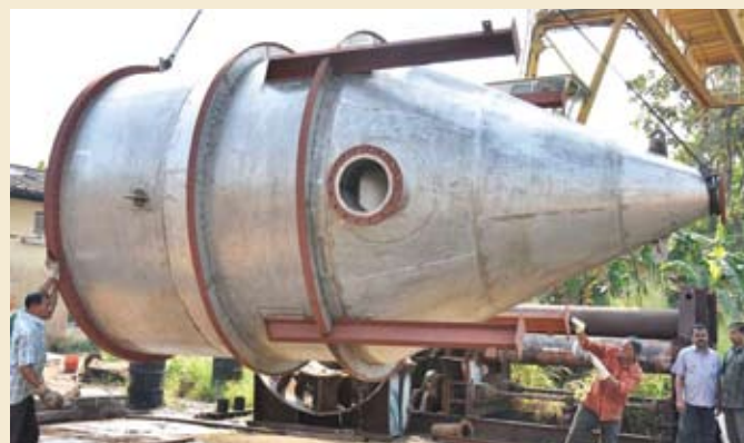
Stainless steel vessel for bag filter-KMML-2011
