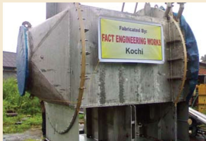
Heat exchanger for VSSC
