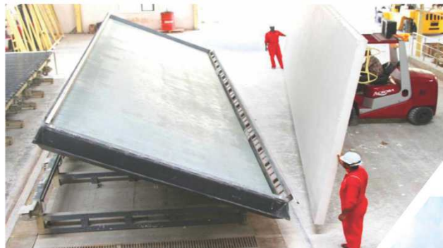
Glass Reinforced Fibre Gypsum Panel, FRBL, Ambalamedu, Cochin
